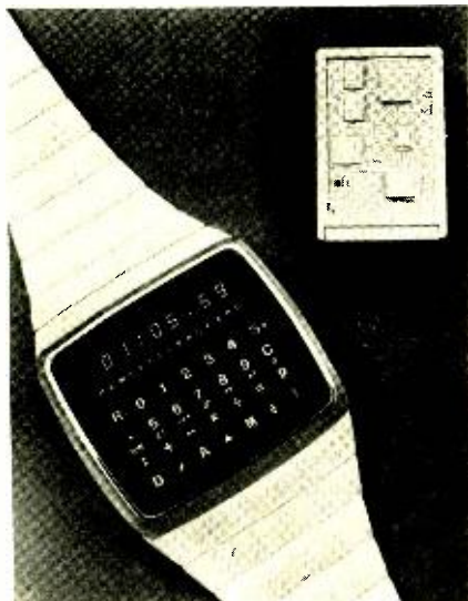
CALCULATOR/WATCH has 28 keys to perform more than 36 different operations using six basic interactive functions.
