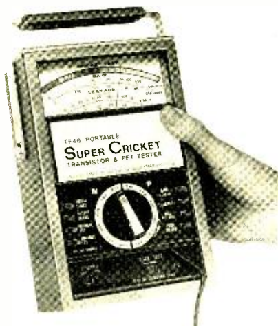
SENCORE TESTER TAKES ITS "CRICKET" name from fact that instrument "chirps" to indicate good transistor. Several models let you measure parameters too.
